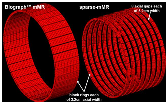
Fig. 1: Visualization of Siemens Biograph™ mMR and sparse-mMR with 8 block rings.
