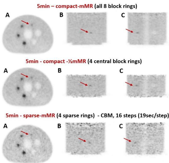
Fig. 3. (A) Transverse, (B) coronal, and (C) sagittal views of 3D PET images of the NEMA image quality phantom reconstructed from 5min list-mode PET scans using (1<sup>st</sup> row) the compact-mMR and (2<sup>nd</sup> row) compact  $\frac{1}{2}$ mMR configurations in stationary acquisition mode and (C) the sparse-mMR configuration in CBM mode with constant bed speed.
