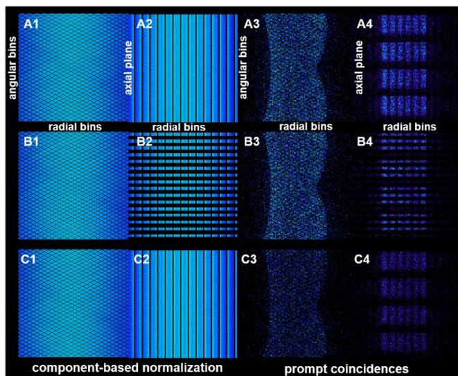
Fig. 2. Two sinogram views of (1<sup>st</sup>-2<sup>nd</sup> column) component-based normalization factors and (3<sup>rd</sup>-4<sup>th</sup> column) prompts counts from 5min scans, corresponding to (A) the compact-mMR configuration, (B) the sparse-mMR configuration without CBM and (C) the sparse-mMR configuration with CBM mode of 6.4cm bed translation and constant bed speed.
