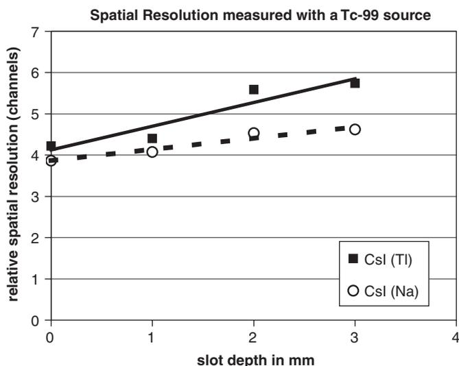
Fig. 4. Spatial resolution of CsI(Tl) and CsI(Na) partially slotted scintillators as a function of slot depth, when an capillary filled with Tc<sup>99</sup> is placed in 5 mm distance from collimator surface.
