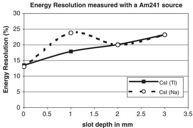
Fig. 3. Energy resolution of CsI(Tl) and CsI(Na) partially slotted scintillators as a function of slot depth, when an Am<sup>241</sup> source is used.
