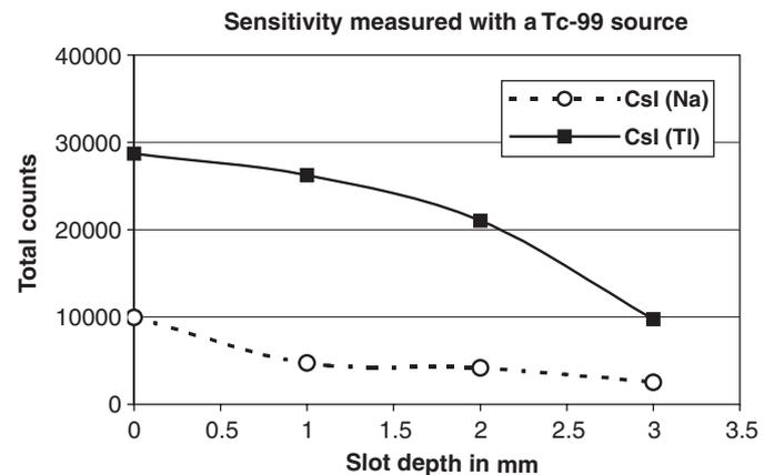
Fig. 1. Sensitivity of CsI(Tl) and CsI(Na) partially slotted scintillators as a function of slot depth.
