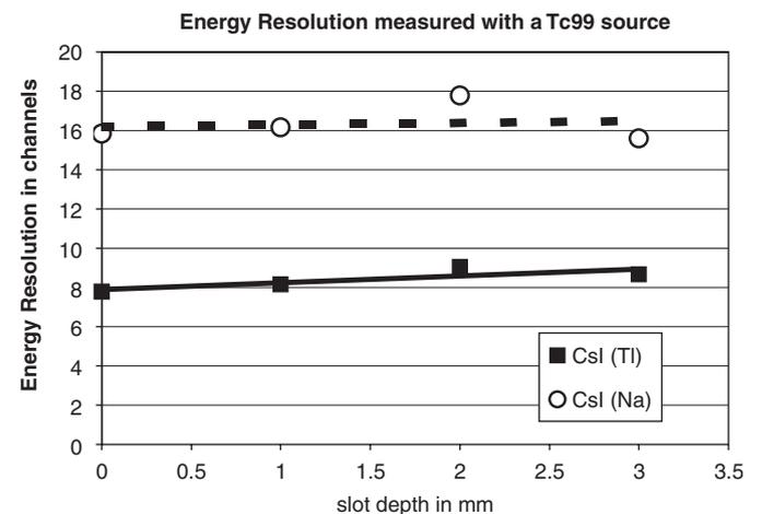
Fig. 2. Energy resolution of CsI(Tl) and CsI(Na) partially slotted scintillators as a function of slot depth, when a point like Tc<sup>99</sup> source is used.
