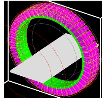
Fig. 2. Biograph 2 geometry model using cylindrical PET system in GATE.
